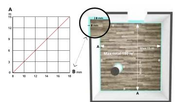
The size of the movement joint in mm is calculated using the formula: 2 mm x 3-meter floor area. The size of the movement joint should never be less than 8 mm. Remember to remove the spacers after installation is done and complete!
